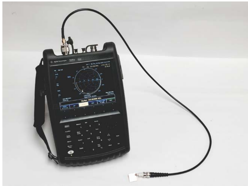
Figure 28. VNA with mussel shell parallel plate capacitor
